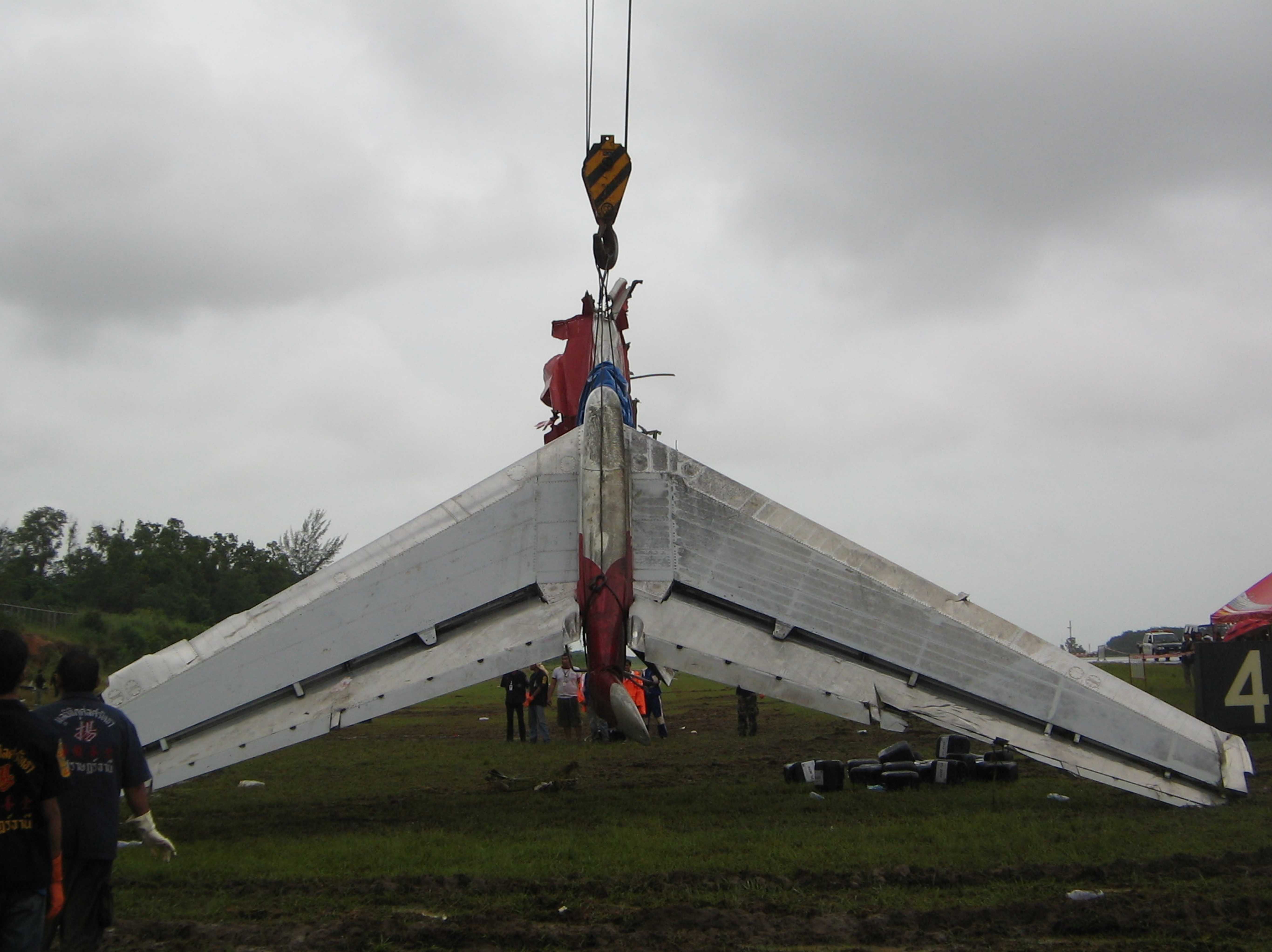
Photo 2 - Aircraft Tail Section During Recovery (Boeing photo)
